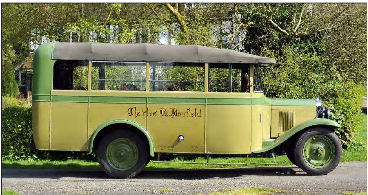
Built by B&T in 1929 and now restored, this 14 seater coach with canvas roof is based on a Chevrolet chassis. Later, of course, General Motors introduced the “Bedford” marque to commercial vehicles made in the UK.
